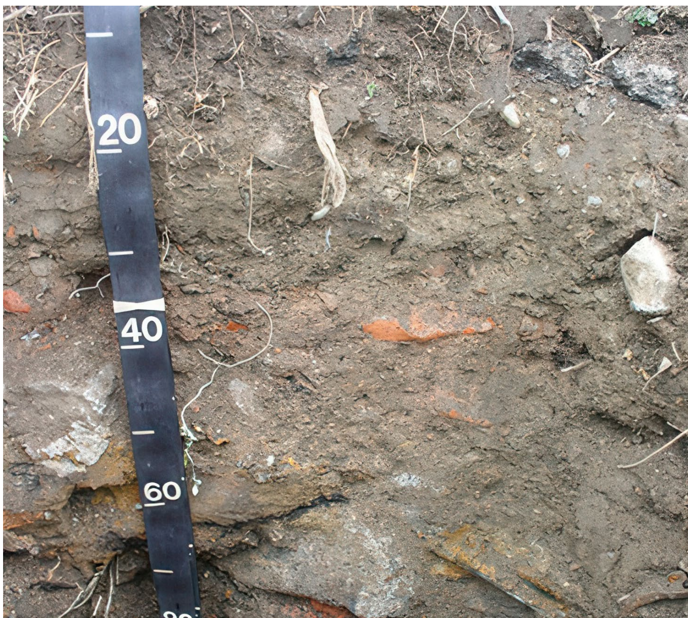
HAHT soil profile showing debris including brick, concrete, wire, steel, and asphalt. 185
